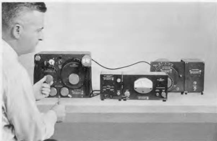
Figure 14. Photograph of system shown in Figure 14. Bridge is the Type 1606-A RF Bridge.
